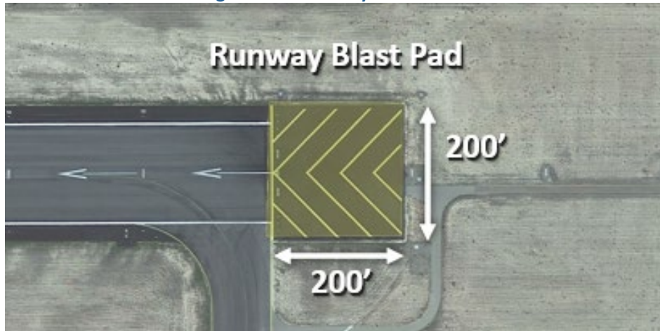
Figure 4-27: Runway 25 Blast Pad
