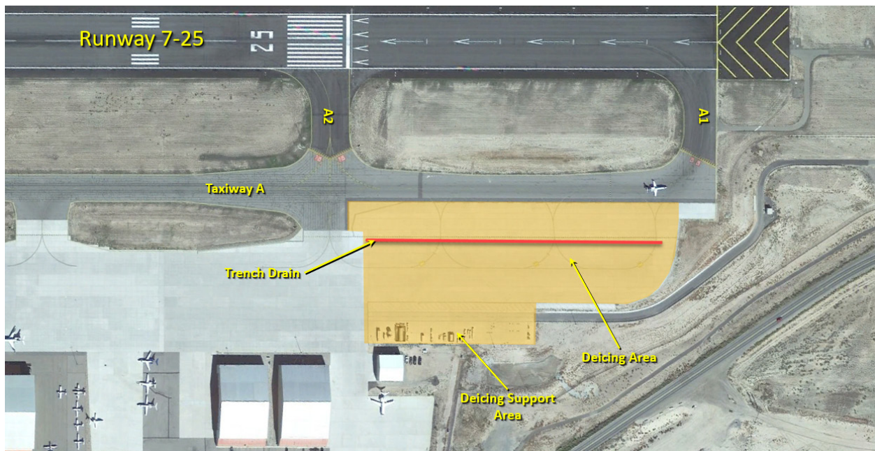
Figure 2-11: Aircraft Deicing Areas and Corresponding Trench Drains
